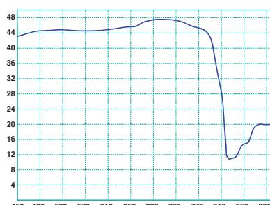
Gain (x: frequency MHz, y: ISO dBi gain) and Pattern (@600MHz)
